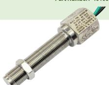
ATEX/IECEx certified explosion proof magnetic speed sensors for Class I, Division 1, Group A, B, C, & D hazardous areas. Designed for use in atmospheres containing acetylene, flammable gas, flammable liquid-produced vapor, or combustible liquid-produced vapor.
